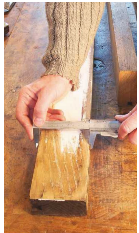
▲ Pic.5 Vernier callipers are a must if using odd timber sizes
